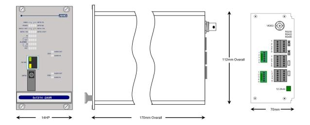
The **AMG5914-2A9R** is a rackmount one channel video receive unit designed to receive 1 video signal and transmit and receive 2 data signals, 2 audio channels plus 8 bi-directional alarms and also provides full duplex 100Base-T Ethernet connectivity over one Singlemode optical fibre.
